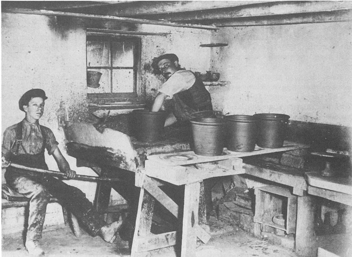
Fig. 51. The potter in this picture, taken in 1927, is Herbert Bailey and his assistant is Harold Churchill who still lives in Verwood. They are making flower pots on the primitive pole-operated wheel.
