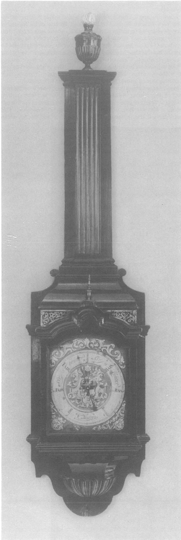
Plate 1. Wheel barometer by William Bastard in ebonised case. Height (including finial) 50"; maximum width 12"; maximum depth 4".
