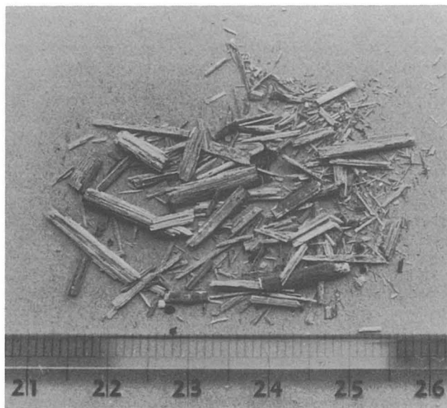
Plate 22. The spacer two weeks after it had split. Scale in mm.
