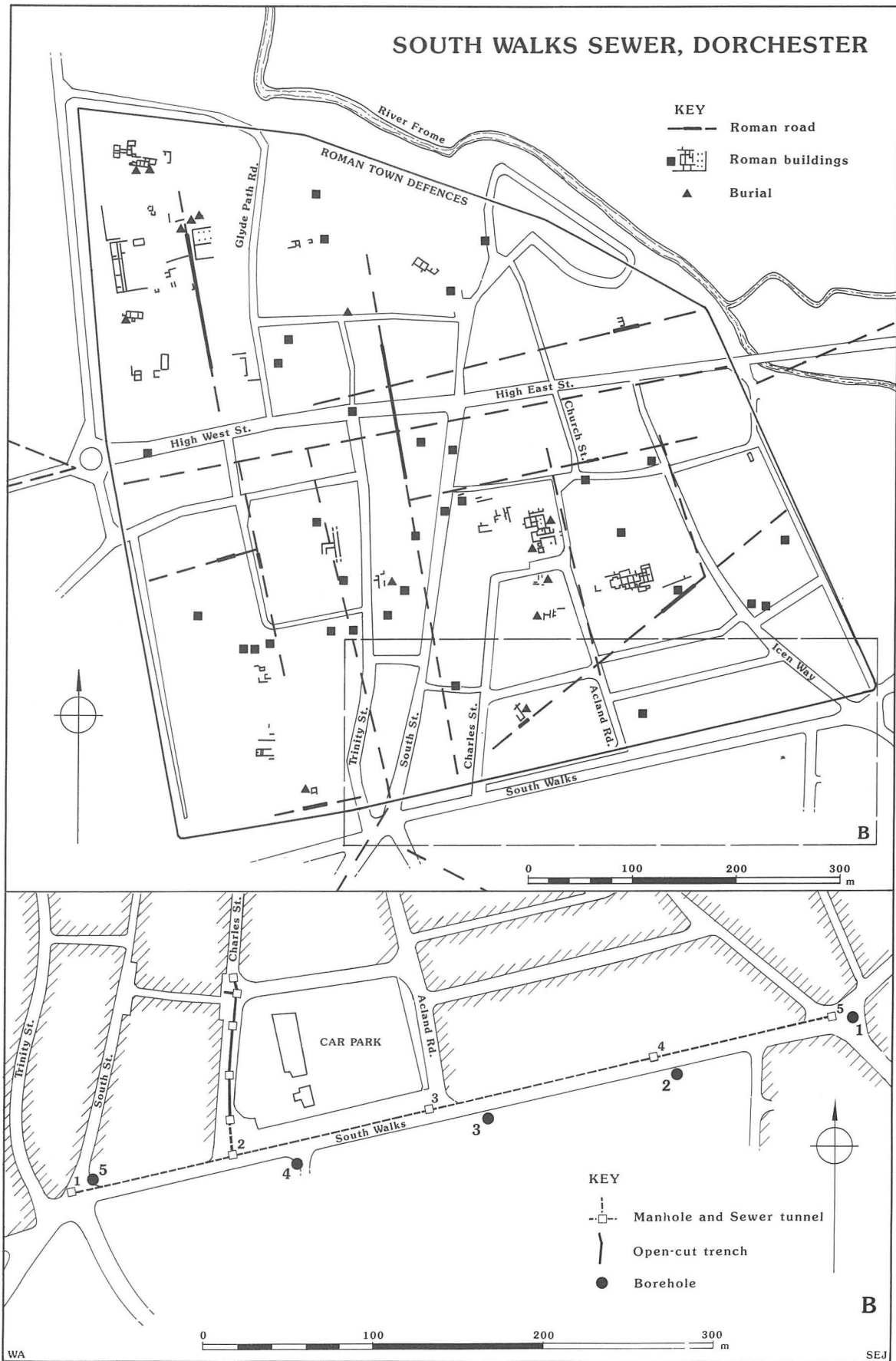
Fig. 1. Location of tunnel and open-cut sewer trenches, and preliminary boreholes, shown in relation to Roman features.
