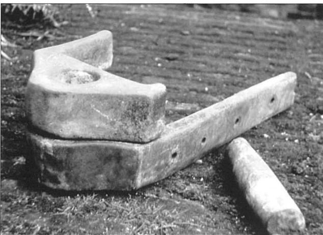
Figure 5: The broken pintle. (Reproduced with the permission of Rodney Alcock)
