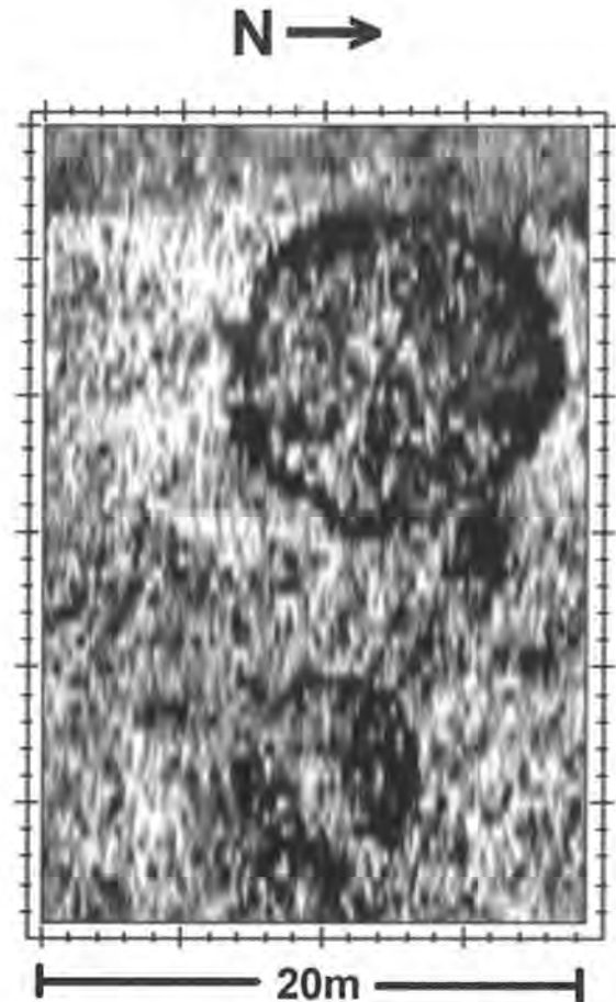
Figure 6: Radar plot of crop marks – horizontal slice at 8.29ns (approx. 0.85m)
